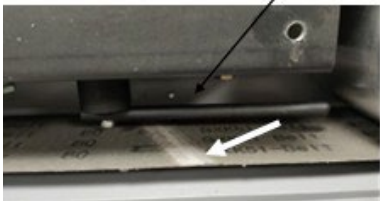
Belt Tension Lever Closed - Pull To Slacken
