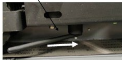
Belt Tension Lever Open - Push To Close
