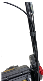
(b) Securing the control cables using the cable clips.
