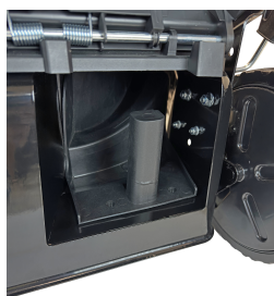
(a) The fitted mulching plug, without the grass catcher fitted to the lawnmower.
