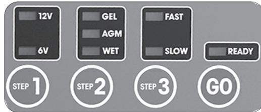
**Step 1** - Select the correct voltage of the battery.
