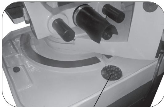
Machine base filter
